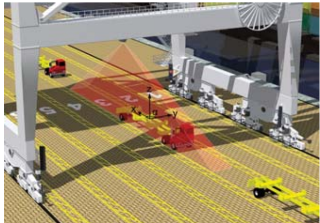
Truck Positioning System – Position acquisition/target position measurement
